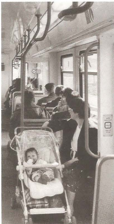
Spaces with pull-down seats cater for mothers with push-chairs and for passengers with luggage.
