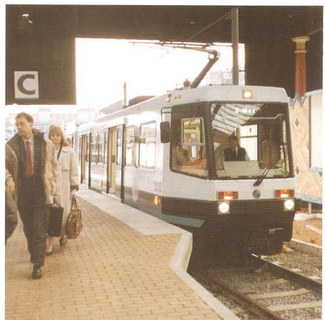
The close fit between the vehicle doorway and the platform is clearly visible, a design feature of the whole system to make it readily accessible to the disabled.
