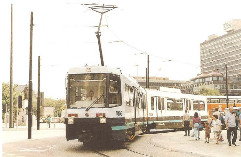
The vehicle easily negotiates a 25m radius curve on the street section.
