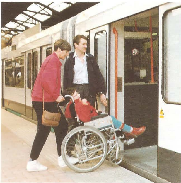
The close fit between the vehicle doorway and the platform is clearly visible, a design feature of the whole system to make it readily accessible to the disabled.
